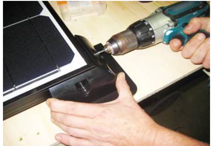
2. Attaching ABS corner mounts to solar panel.
