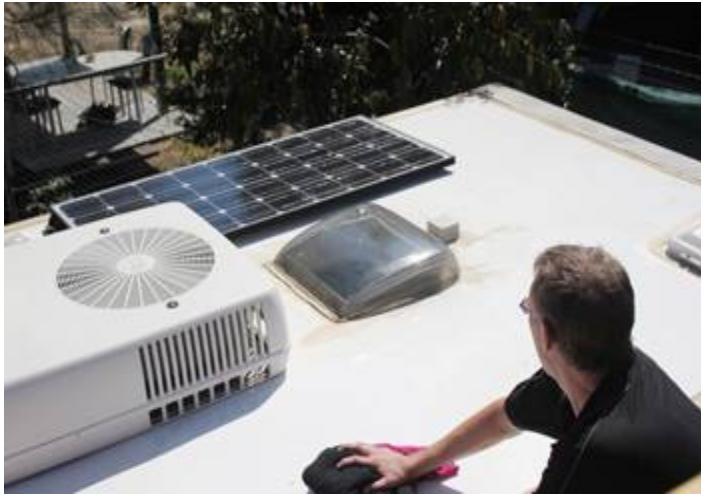
1. Praparing vehicle surface for solar panel.
